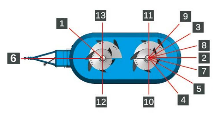
\* Windows no 10, 11, 12, 13 - make the wagon wider by 20 cm on each side In model FXXL 1400 HD, windows no 1, 4 and 9 make the mixer wagon wider by 4 cm on each side
