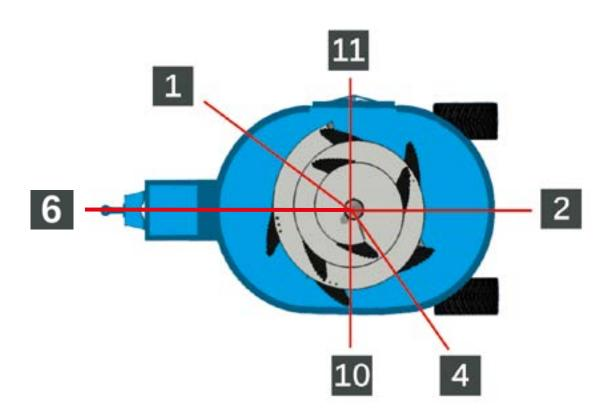
\* Windows no 10, 11 make the mixer wagon wider by 20 cm on each side Windows no 1,4 makes the mixer wagon wider by 4 cm on each side
