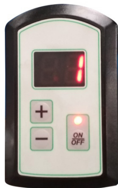
Fig.19. Electronic control of chain floor conveyor speed ARPWM V1.1.
