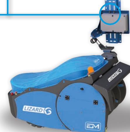
UK EM LIZARD is driven by BLDC brushless motors with planetary gearboxes, which ensures maintenance-free operation. The biggest advantage is a modular auger made of highly abrasion-resistant plastics. The patented design of the modular auger makes it possible to shape each module, so that the feed is not only moved towards the cows, but is also perfectly aerated.
