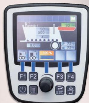
🇬🇧 Electronic control of the chain conveyor
