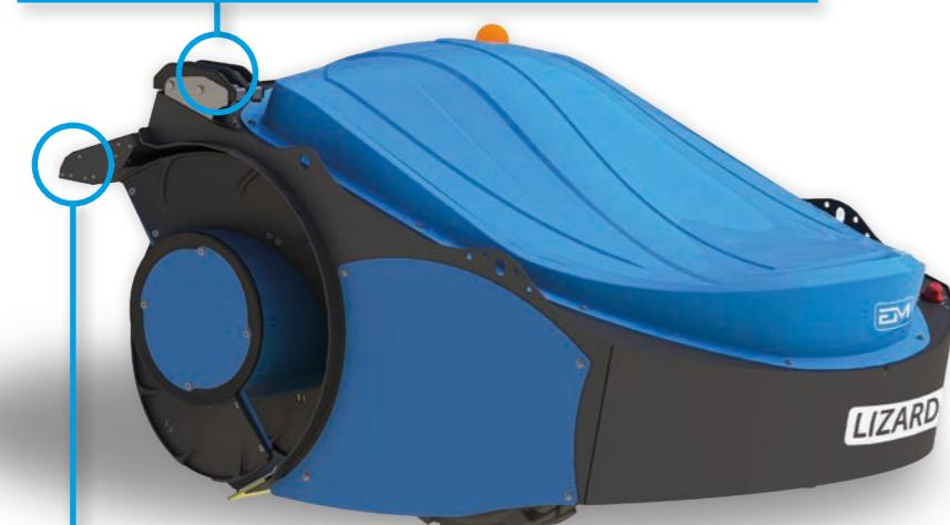
Two-way safety bumper - obstacle detection in front of the robot
