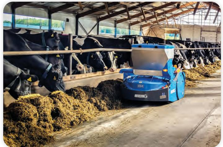
🇬🇧 EM LIZARD is driven by BLDC brushless motors with planetary gearboxes, which ensures maintenance-free operation. The biggest advantage is a modular auger made of highly abrasion-resistant plastics. The patented design of the modular auger makes it possible to shape each module, so that the feed is not only moved towards the cows, but is also perfectly aerated.
