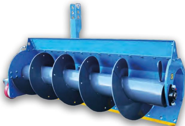
🇬🇧 EM Viper performs two functions: pushes and softens the TMR. This is possible thanks to the use of a spiral. It can be equipped with paddles, which additionally increase the effect of aeration of the fodder. Viper is powered by a 125 cm<sup>3</sup> hydraulic motor and the required capacity for proper operation is 10l/min.
