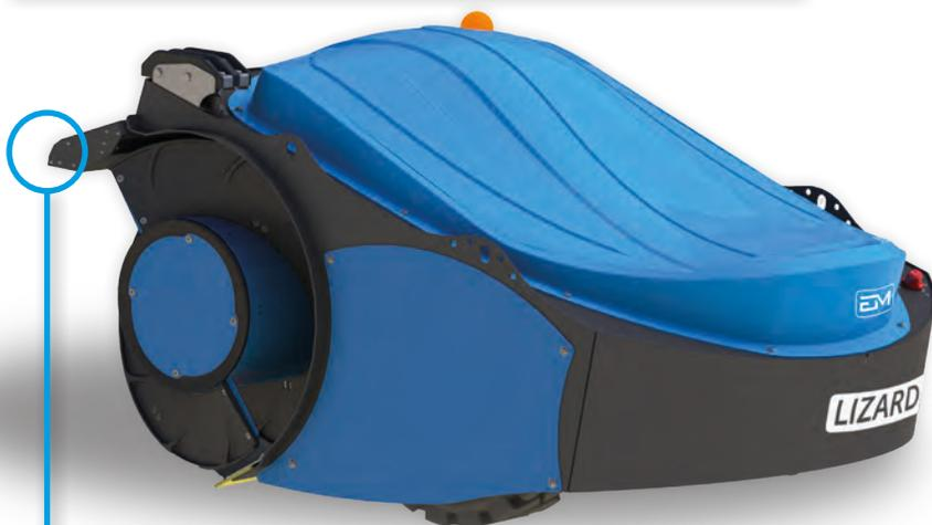
Two-way safety bumper - obstacle detection in front of the robot
